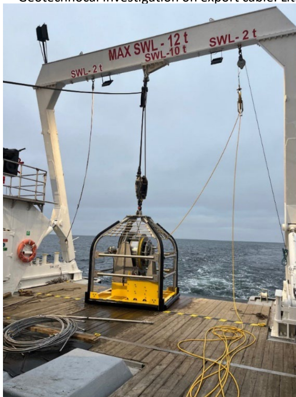
Fig.5. Neptune 5000 CPT rig with power and data cables
